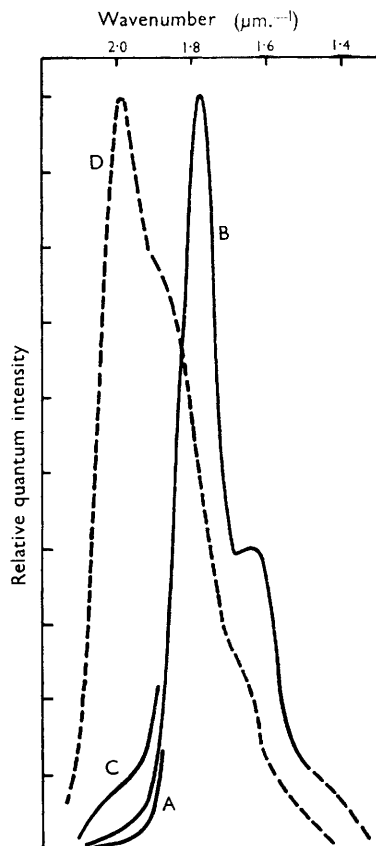
FIGURE. Photoluminescence emission spectra of 2 \times 10^{-4} M benzil in perfluoromethylcyclohexane. (A)(B)(C) long-lived emission in de-aerated solutions: (A) directly excited by 313 nm. at -19^\circ ; (B) both directly excited (313 nm.) and sensitised by benzophenone (366 nm.) at +20^\circ ; (C) sensitised by benzophenone at +60^\circ ; (D) prompt fluorescence of an aerated solution. Intensity scale of (D) is not comparable with remainder.
